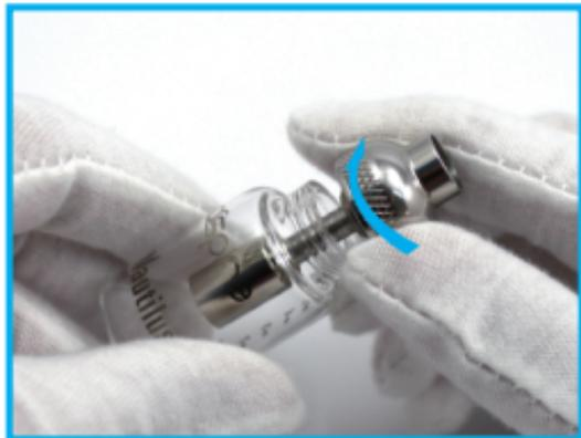
2. Screw the BDC Atomizer into the bottom hardware (make sure the BDC atomizer is snugged down hand tight).
