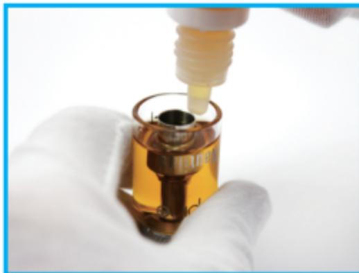
4. Screw the bottom hardware back onto the upper hardware.
